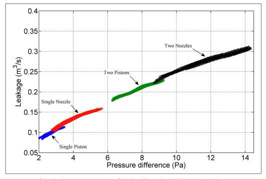
Figure 9: Comparison of the leakage measurement of the building obtained by nozzle and piston units.
