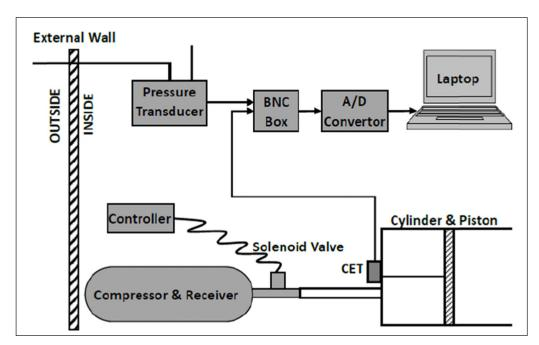
Figure 6: Schematic diagram of pulse technique using piston unit.
