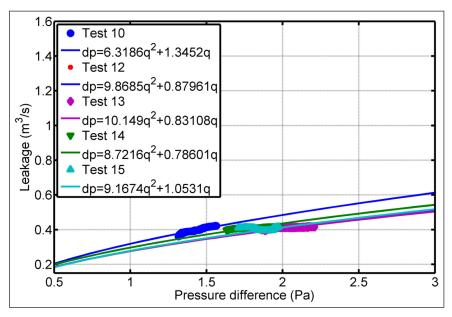
Figure 17: Leakage characteristic and power law fitting when vents were sealed.
