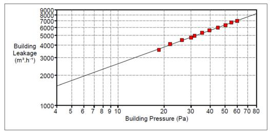
Figure 2: A typical steady state airtightness test (Log-log plot).
