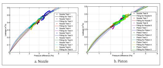
Figure 14: Leakage characteristic measured by piston and nozzle based pulse units.
