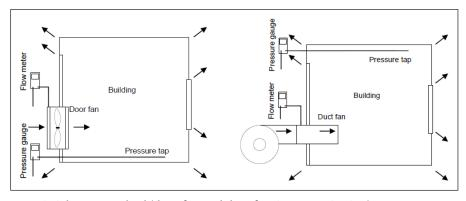
Figure 1: Steady state airtightness method (door fan and duct fan: in pressurisation).
