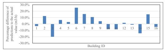
Figure 11: Percentage difference of predictions of  $Q_{50}$  to that measured by BD-M4.
