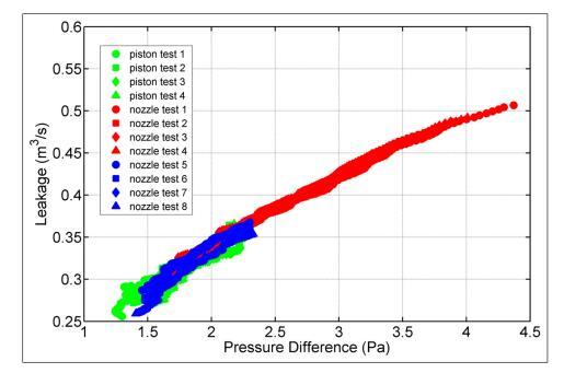
Figure 15: Comparison of results obtained by three nozzle units and three piston units.
