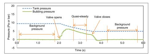
Figure 3: A typical pulse test by a unit with 60 l tank (tank pressure measured in bar, building pressure in Pa).
