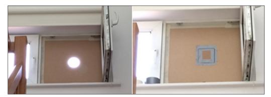
Figure 12: Setup of the known opening in house No. 8.
